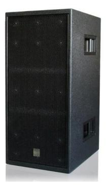
The sound reinforcement system shall hold two low-weight neodymium 21-inch drivers, each powered by a 2500W class-D amplifier. The maximum peak output of the total system shall be 140dB at 1m. The system shall be switchable between full range or the 25-60Hz frequency range. The systems coverage angle shall be omni-directional.
