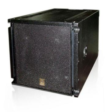
The sound reinforcement system shall hold one low-weight neodymium 18-inch driver, powered by a 1000W amplifier. The maximum peak output of the total system shall be 132dB at 1m. The system shall reproduce the 30-60Hz frequency range. The systems coverage angle shall be omnidirectional.
