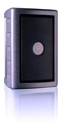
The sound reinforcement system shall hold a 1" HF driver and a 10" driver mutually mounted on a waveguide. Powered by a 600W and 300W amplifier, the maximum peak output of the total system shall be 125dB at 1m. The system shall have a 50Hz-20kHz frequency range. The systems shall have a coverage angle of 100 degrees horizontal and 40 degrees vertical with a soft roll-off.
